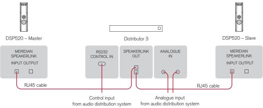
Each module in the Distributor 3 can distribute a digital or analogue source to a pair of Meridian DSP loudspeakers.
