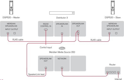
One of the three modules in a Distributor 3 can be used to connect a pair of Meridian DSP loudspeakers to a streaming system, via a Meridian component such as the Media Source 200.
